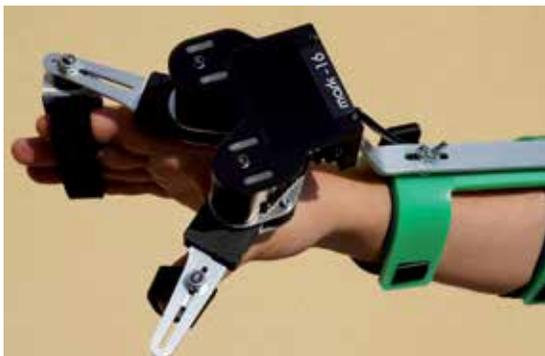
Figure 5b. Mark-16 in motion – extended hand.
