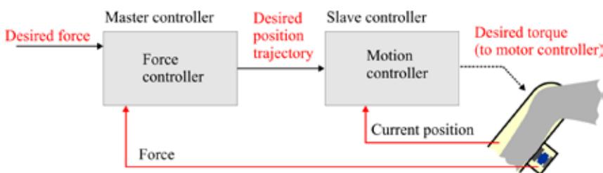
Figure 8. Basic structure of the force controller.
