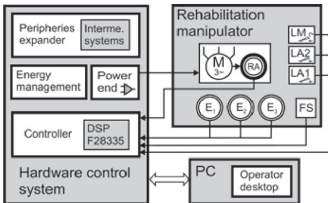
Figure 5. Schematic diagram of hardware control system.
