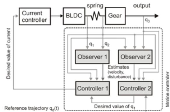
Figure 6. Basic structure of the motion controller.
