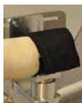
Figure 2. Shine fastening unit: a) CAD model: 1 – shine fastening with force measurement unit, 2 – shine model, 3 – fixing band, 4 – manipulator’s arm, 5 – manipulator’s rotational axis; b) picture of shine fastening unit with lower limb medical model.
