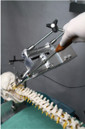
Figure: Elements of the system for spine surgery: M- marker of the optical tracking system, R- robot, PS- arms of the passive structure
